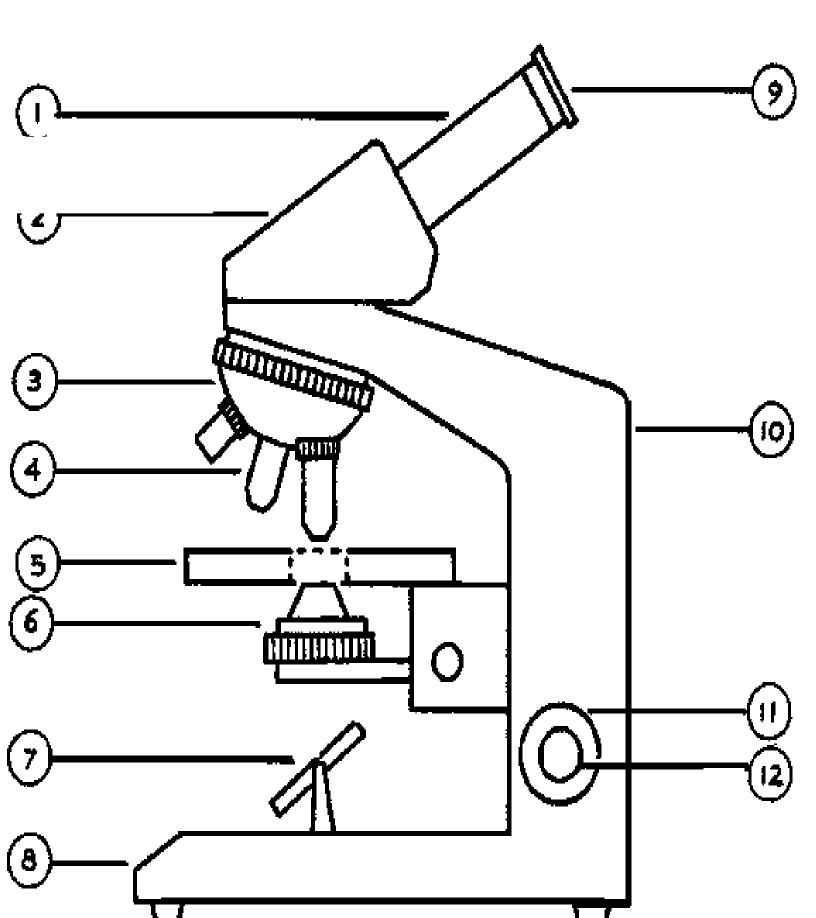
WORD BANK (Use for BOTH the labeling of the microscope as well as the fill-in the blank questions) Eyepiece Body tube Objectives Nosepiece Stage Diaphragm Light Source Base Spring (Stage) Clips Arm Fine Adjustment Knob Coarse Adjustment Knob
